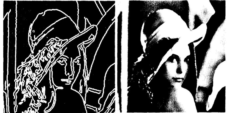
Stephane Mallat and Sifen Zhong at the Courant Institute used a maxima chain representation (left) based on wavelet analysis to compress data from a digitized image. The reconstructed image (right) is virtually indistinguishable from the original.
